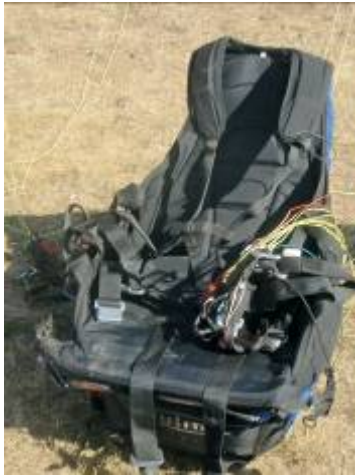
Harness with back protection - This device holds the pilot to the paraglide and allows him or her to sit down comfortably while in the air.
